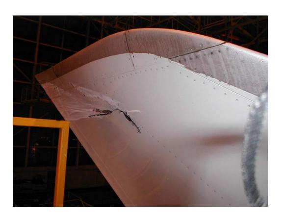
Remove winglet, inspect attachments and despatch to CDL with performance penalties
