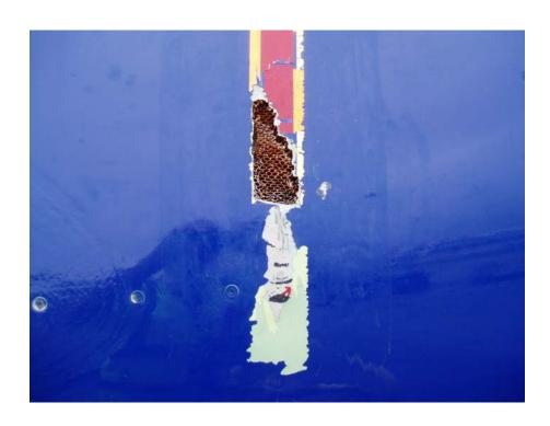
Temporary repair at hangar –delay service
